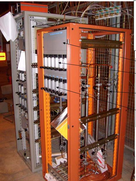
Gas re-circulation rack (from ATLAS). During the first phase of the test we will use the system in open mode. The gas from the RPC will be send to the filters rack and then vented.
