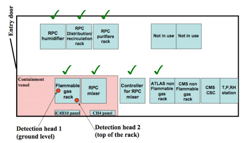
All pipes and racks have been tested for leak tightness (30' at constant P)
