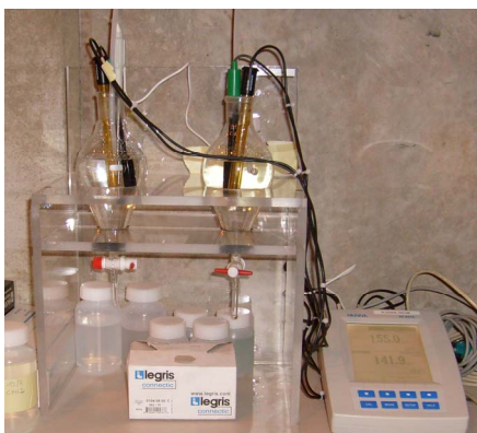
Fig. 3. Picture of the Hanna double channel analysis station used for the measurement of the fluoride production. The two bubblers containing the water used to trap the F^- ions present in the RPCs exhaust mixture are visible.
